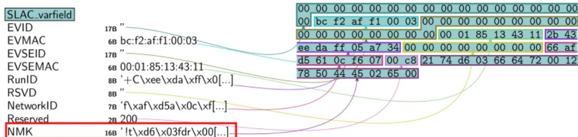
Our PLC can be easily set by changing *slac/pev.ini* profile and used with *pev* tool<sup>2</sup>
